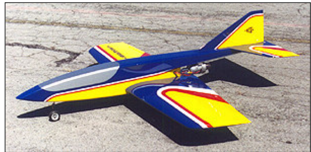
My prototype uses a RAM 500 for power. It's given me some fits during startup, but is a reliable runner once it's going. Other suitable turbines for the R54 are the PST J600, Wren 54, FTE T500, and Simjet 1200. Most of the engines in this 11-14lb thrust class are based on a 54mm compressor, so the model's official name, Reaction 54, is meant to reflect the size turbine for which it was designed.
