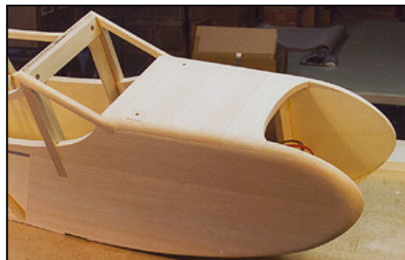
Above - Hatch removed. The hatch is held down at the back using two 10-32 nylon bolts threaded into plywood blocks under the lite-ply. A lite-ply tongue holds the hatch at the front. Below - 1/16" ply hardpoints are imbedded in top of hatch. The fuselage corners have all been sanded round.
