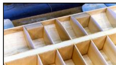
Below: This is a view of the center wing panel, upside-down, with the top LE sheeting, shear webs, and the two wing dowel blocks in place.
