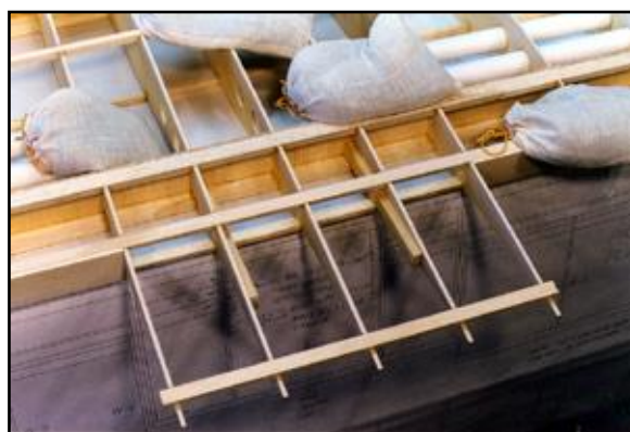
Center Wing Panel, Right-Side Up - with the shear webs and spruce reinforcing sticks in place. Be careful working around those ribs hanging off the table - they're easy to bump into.
