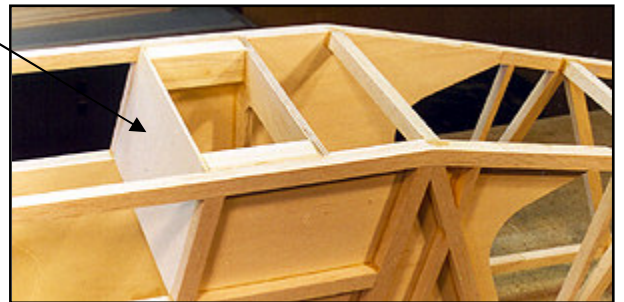
Fuselage Top showing the cabin rear and laminated wing blocks glued in place.
