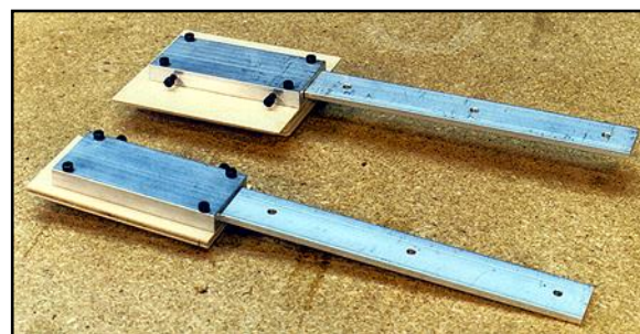
Top: Front Joiner Assembly. Bottom: Rear Joiner Assembly - At this point, the joiners have been fastened to the center section shear webs. Notice the "open" side of the C-channel is positioned against the face of the plywood web.
