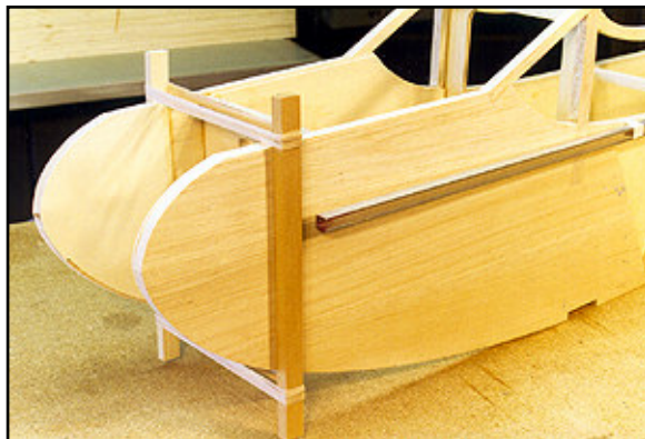
Fuselage Front End shows the stick and rubber band squeezing tool. I used a straight channel of aluminum taped to each side in the cabin area to help visualize and measure that the front end of each side was pulled in equally.
