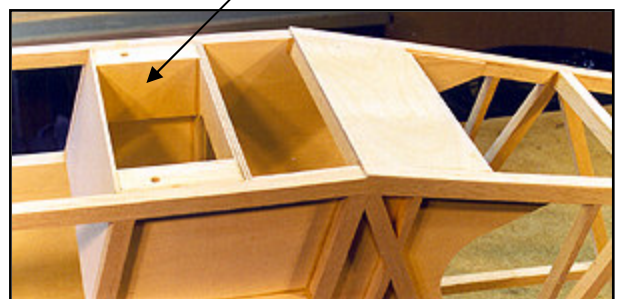
Fuselage Top showing the position of the wing block supports. The wing bolt holes have been drilled and tapped. This photo is a little out of sequence because it shows the plywood fuselage top aft of the wing and the 3/32" balsa caps on the rear fuselage (to be installed in the next section).
