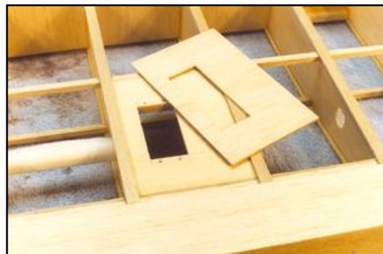
Aileron Servo Mount - with balsa sheeting ready to be glued in place. Note the extra-long cutout in the balsa. The servo flanges should sit flat against the lite-ply, not the balsa.
