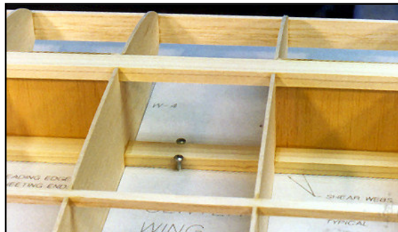
Center Wing Panel - Notice the screws holding the bottom main spar to the table. The front screw needs to be removed before the shear web can be added. Note the grain of every shear web must be vertical!
