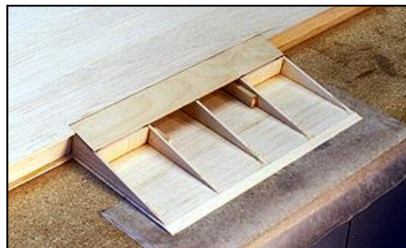
Center Wing Panel, Top View - You can see the bottom center TE sheeting has been beveled to match the rib contour. When the top sheeting is glued on, the glue joint formed between the two sheets will help toughen the wing trailing edge.
